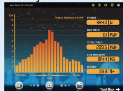
Showing data of Power / Day Yield / Total Yield / CO 2 Emission / Money etc.
